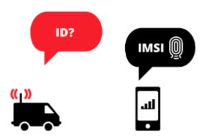
In successive generations, ie 3G and 4G LTE, the attack gets more complex. The attacker with his fake BTS would try to spoof the connection request and act Man-in-the-Middle. Then the service would get downgraded to the non-encrypted GSM instead of more secure 3G/4G
